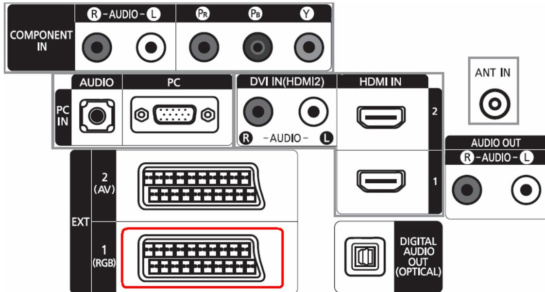
Connect the SCART adaptor to the video output of your TV. Connect one side of the composite cable to the SCART adaptor and the other side to the AV1 Input “AV1 IN” of your CM3G/P/PP.
