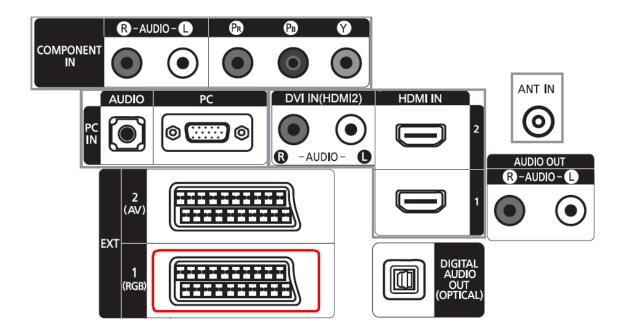
Connect the SCART adaptor to the video output of your TV. Connect one side of the composite cable to the SCART adaptor and the other side to the AV Input "IN" of your CM3PVRD.
