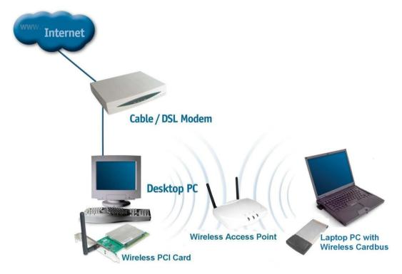
Please note that this type of installation requires that your ISP (Internet Service Provider) provides you a static IP address for each computer and the Access Point on your network. Please refer to the manual that came with your Access Point to determine its configuration.
