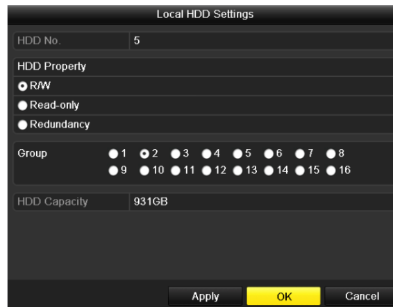
Figure 10-13 Local HDD Settings Interface
