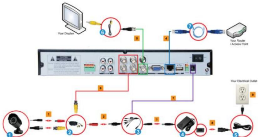
1. Connect the BNC Connector and the Power Connector of the CCTV Cameras(1) with Camera Cables(2).
