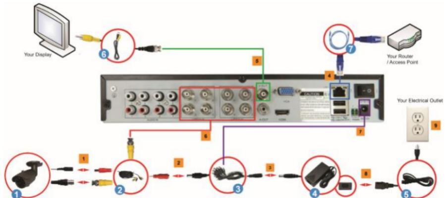
1. Connect the BNC Connector and the Power Connector of the CCTV Cameras(1) with Camera Cables(2).
