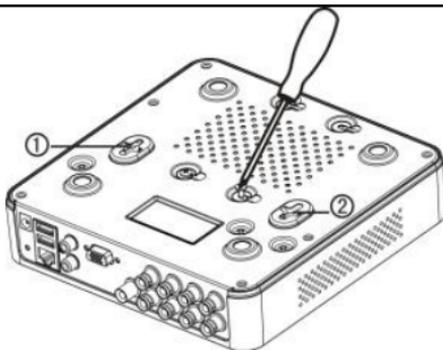
4) Re-install the cover of the DVR and fasten screws.
