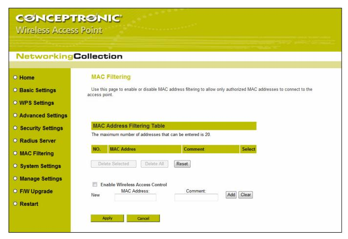
This page contains two parts of MAC filtering information. All allowed MAC addresses will be listed in upper part, and you can add new MAC addresses by components in lower part.
