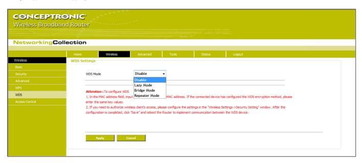
WDS (Wireless Distribution System) is used to expand wireless coverage area. This Router provides three modes: Lazy, Bridge and Repeater.
