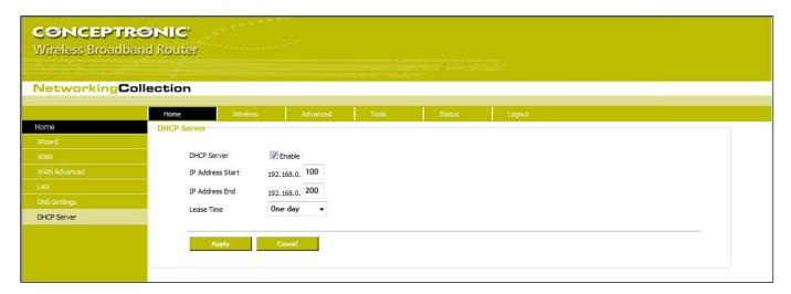
A DHCP (Dynamic Host Control Protocol) is to assign an IP address to the computers on the LAN/private network. When you enable the DHCP Server, the DHCP Server will allocate automatically an unused IP address from the IP address pool to the requesting computer in premise of activating "Obtain an IP Address Automatically". So specifying the starting and ending address of the IP Address pool is needed.
