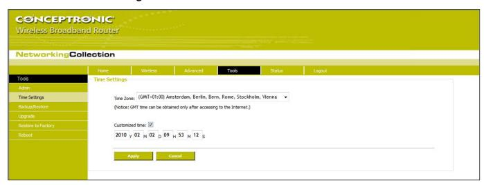
This section is to select the time zone for your location. If you turn off the Router, the settings for time disappear. However, the Router will automatically obtain the GMT time again once it has access to the Internet.
