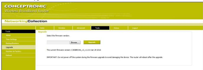
The Router provides the firmware upgrade by clicking the "Upgrade" after browsing the firmware upgrade packet which you can download from <a href="https://www.conceptronic.net">www.conceptronic.net</a>.
