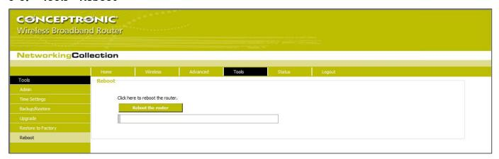
Rebooting the Router makes the settings configured go into effect or to set the Router again if setting failure happens.
