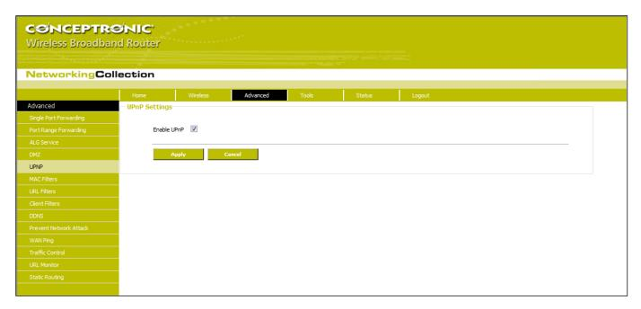
It supports latest Universal Plug and Play. This function goes into effect on Windows XP or Windows ME or this function would go into effect if you have installed software that supports UPnP. With the UPnP function, host in LAN can request the router to process some special port switching so as to enable host outside to visit the resources in the internal host.
