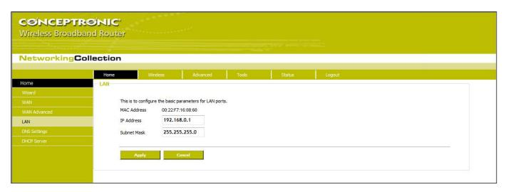
LAN Settings are for the basic TCP/IP parameters of LAN ports.
