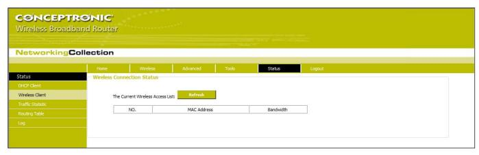
This page shows wireless client's connection status, including MAC address, Channel bandwidth, etc.
