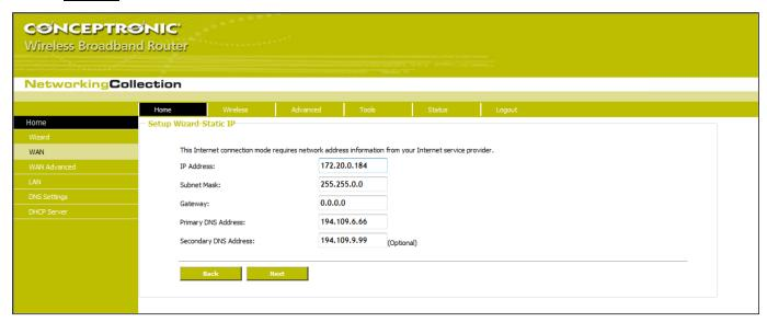
In this screen, fill the network address information from your ISP in the IP Address, Subnet Mask, Gateway and Primary DNS server fields and click "Next".
