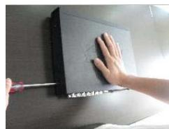
⑥ install the screws on both sides of shell
