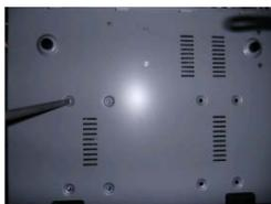
④ fix the screw of hard disk
