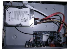
③ connect hard disk and mother board
