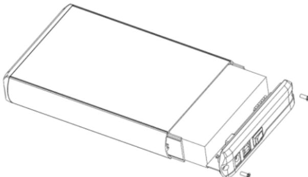
**English** : Connect the hard disk to the SATA connector. Insert the hard disk into the enclosure. Replace the back panel and fix it with the screws which were removed in step 1.
