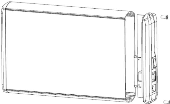
**English :** Remove the screws on the backside and remove the back panel.
